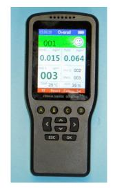
MGC Air Quality Monitor is designed to help identify the level of contaminates, particles and pollution in the air, both in the home & outside. The monitor measures particles which consist of mould spores, fungi spores, pollen, dust, organic matter & chemicals suspended in the air
